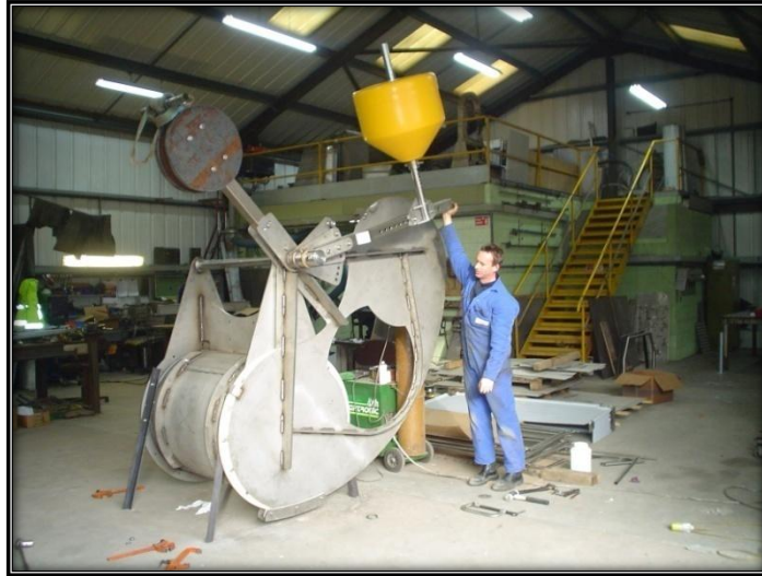
The above image shows the valve being tested in the closed position. This is how the valve would appear during high-tide.
