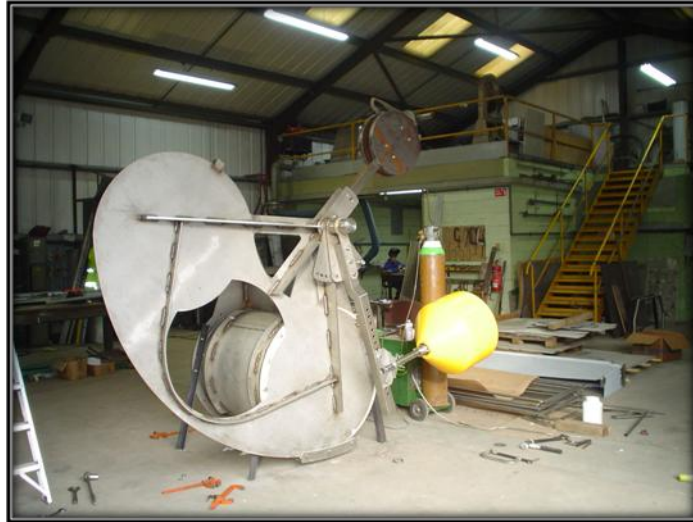
The image above shows the valve being tested in its closed position. This is how the valve would appear during low-tide.
