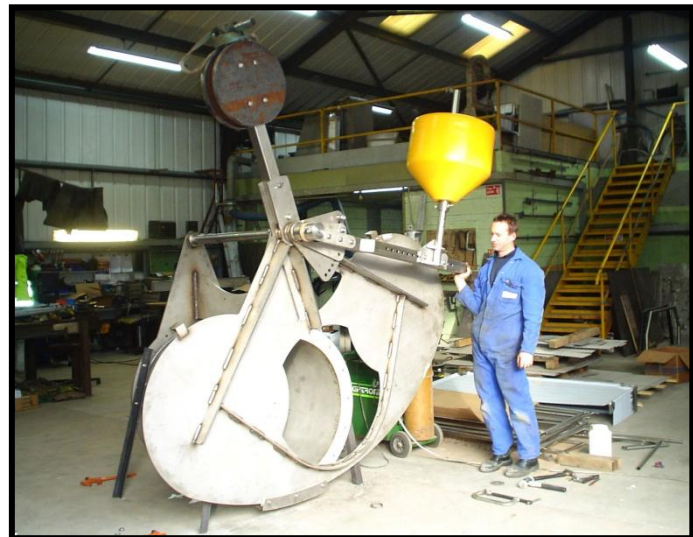
The image above shows the valve being tested in the half-closed position. This is how the valve would appear during mid-tide.
